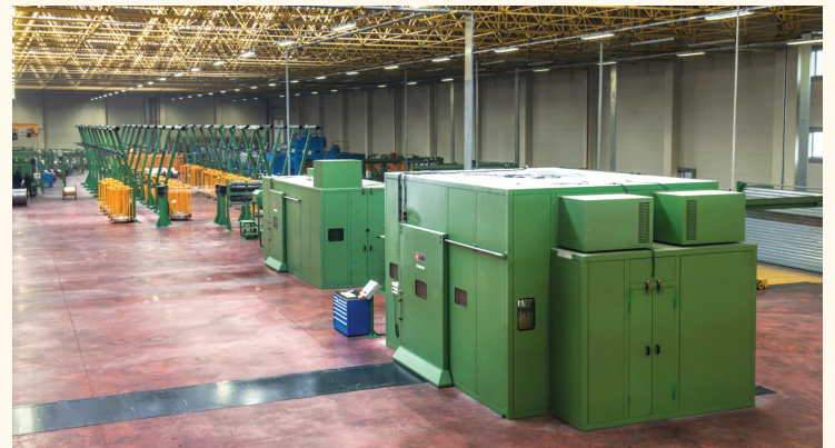
SETIC 2000 mm Large Double Twist Strander (TC2000-4M)
