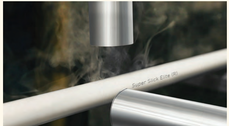
Encore Wire marks a wide variety of cables at its facility in Texas. The LEIBINGER JET RAPID can mark cables at speeds of up to 3,280 ft/min. Source: Paul Leibinger GmbH & Co. KG
