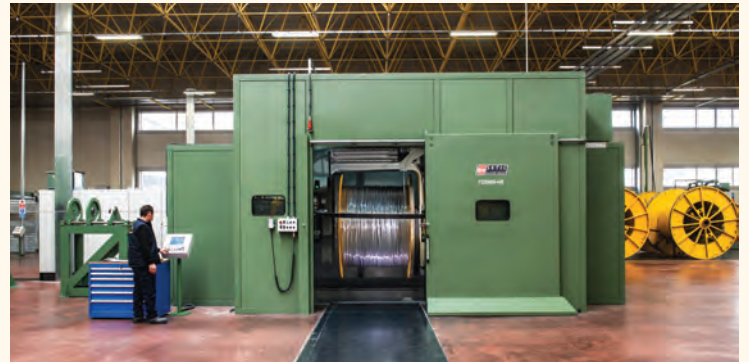
2000 mm Large Double Twist Strander (TC2000-4M)
